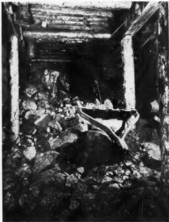
TOOTHED SCRAPERS , 42 inches wide, pulled by 15 horsepower double drum air hoists are used to remove broken ore. Broken ore is pulled into footwall transfer raises. The toothed scraper was developed to dig into the steeply banked muck pile full of boulders against the face and to pull load over the rough bottom. Note the teeth at top of scraper. Teeth are on a reversible back plate which is turned 180° when one set of teeth is worn out. Tail sheave is hooked firmly into log mat.
